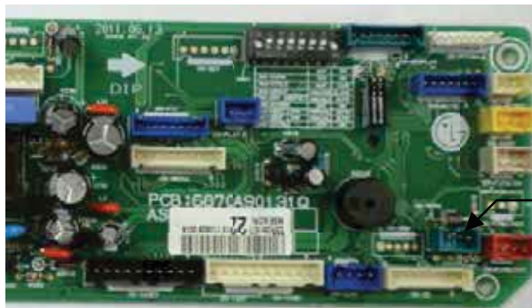
CN-REMO: Remote controller connection
